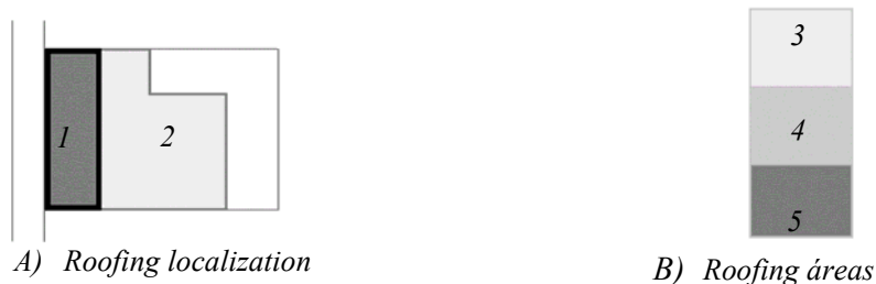
Figure 1. Roofing sketch with localization and coatings. In A): the number 1 is the monitored roofing and the number 2 is the house. In B): the number 3 has white impermeable painting; the number 4 has white acrylic painting and the number 5 has the natural tile color on the monitored roofing.
