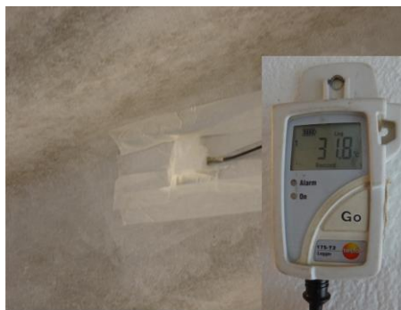
Figure 5. Surface temperature sensor under tiles and mini logger.
